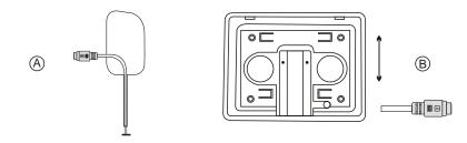
Note: Installing Methodof main cable assembly 1.Reeve the main cable assembly through (or beside) the head rest support tube. 2.Secure and protect the cable assembly from damage when the head rest is adjusted.
